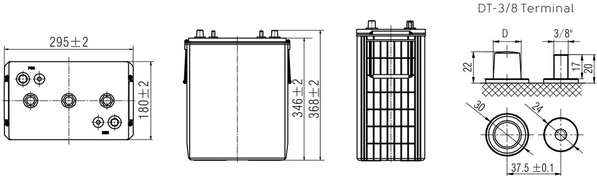
Note: D:Positive  $19.5_{-0.3}^0$ , D:Negative  $17.9_{-0.3}^0$ ; Terminal Torque Values in-Ib(Nm) :176-203(20-23)
